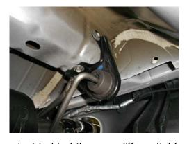
3) Using a 13mm wrench, unbolt the two hangers just behind the rear differential from the cross member. Now, with the help of an assistant, carefully lower the center stand and slide the exhaust system forward and out of the rear hanger mounts. Lower the system to the floor leaving the front hangers attached. Finally remove the two hanger mounts at the rear of the vehicle from the frame using a 13mm wrench. As you remove them, place them with the factory muffler from the corresponding side.
