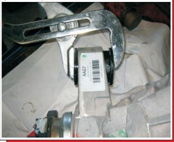
2. You will need to press the old bushings out. Using one of these process (See Picture Below)
