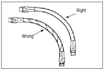
Avoid installing the hose in a twisted position. This can weaken your assembly and loosen fitting connections when under pressure.
