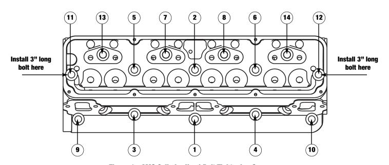
Figure 1 - AMC Cylinder Head Bolt Tightening Sequence (Tighten in four steps: 30, 40, 50, 65-70 or 30, 60, 90, 100-110 ft/lbs)
