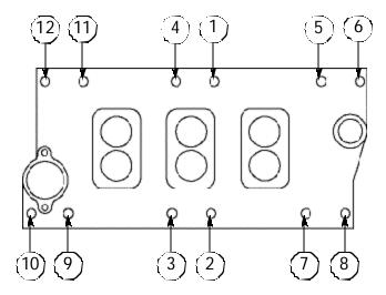
Figure 1 - 262-400 c.i.d. Small Block Chevy Torque Sequence Torque Bolts to 25 ft/lbs.
