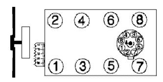
Figure 2 - 262-400 c.i.d. Small Block Chevy Firing Order Firing Order: 1-8-4-3-6-5-7-2 Turn Distributor Counter-Clockwise to Advance Timing
