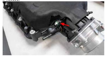
81. Apply 0-ring lube to the 0-ring on the EVAP solenoid and install onto the supercharger manifold using the factory
