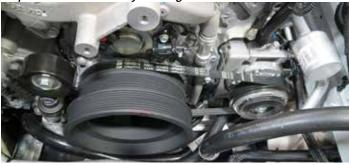
56. Install the factory accessory drive belt using the routing diagram below.
