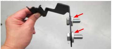
61. Using a 13mm socket, remove the ground strap from the engine block. Location is directly above the A/C compressor.
