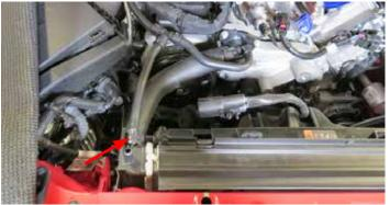
33. Using a hose clamp removal tool, detach the lower radiator hoses. 2017 model year Camaros only have drivers side lower hose. *NOTE: The clamps may not come off because of adhesive. Simply compress the clamp and pull the hose simultaneously.*
