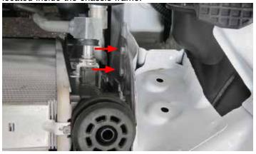
60. Install the water pump assembly onto the water pump bracket. Using the washers from hardware Bag #2 and the factory chassis bolts, mount the water pump bracket to the frame in the location where the chassis bolts were removed. TIP: A secondary wrench may be required to hold the nut located inside the chassis frame.
