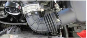
118. Using a razor blade or equivalent, remove the 90° fitting from the factory air inlet PCV hose. Connect the fitting to the supplied air inlet PCV and attach the straight quick connect to the air inlet and the 90° quick connect to the center PCV junction.
