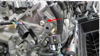
63. Install the supplied tensioner bracket to the provisions on the cylinder head and engine block using two (2) M10 x 100mm bolts and two (2) M8 x 55mm bolts supplied in hardware Bag #1. Torque M10 bolts to 32 ft-lbs and M8 bolts 22 ft-lbs.
