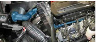
108. Remove the fittings from the factory driver side PCV hose and install into the provided 3/8" hose. Route the hose from the oil separator, around the front coil for cover clearance. Then route the hose around the rear of the manifold toward the driver side PCV junction.
