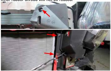
86. Using a 1.75" hole saw, drill a hole into the center of the upper portion of the shroud. Using a cutting tool, remove some material from the center of the shroud opening as shown.
