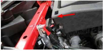
121. Route the EVAP connectors on the supplied water pump harness towards the EVAP solenoid. Install the water pump harness in-between the mating connectors on the EVAP solenoid and factory harness. TIP: Note connector orientation..
