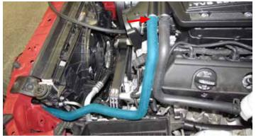
98. Using two (2) 3/4" hose clamps from hardware Bag #2, secure the Surge Tank to Manifold hose to the surge tank and rear water cross over barb.
