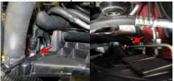
34. Remove the retaining clip securing the transmission cooler line to the radiator and remove the transmission cooler line. *NOTE: Be extremely cautious not to drop or lose this clip. Keep the clip in a safe place to be re-installed later.*
