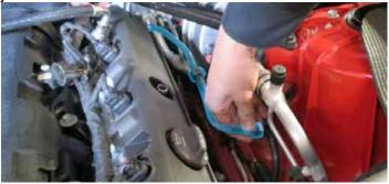
23. Disconnect EVAP connection. Using a 10mm socket, remove ten (10) bolts securing the intake manifold to the cylinder heads. Carefully remove the intake manifold assembly.
