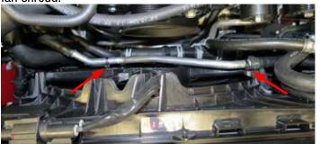
36. Remove two (2) bolts securing the electric fan to the radiator using a 10mm socket. Carefully remove the electric fan assembly.
