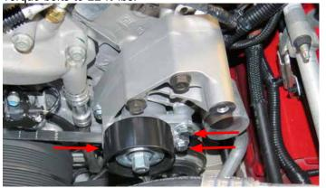
66. Install the larger grooved idler pulley to the FEAD bracket. Torque bolt to 22 ft-lbs.
