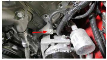
62. Disconnect the engine harness located on the front of the driver side cylinder head. Using a 13mm socket remove the bolt securing the harness to the head.
