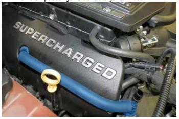
113. Connect driver side pcv hose through the hole in the coil cover.
