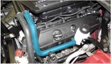
99. Using a 3/4" hose clamp from hardware bag #2, secure the Water Pump to Surge Tank hose to the surge tank.
