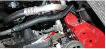
35. Using a panel puller, remove the coolant lines from the fan shroud.
