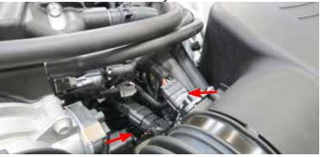
117. Using the supplied worm clamps, secure the inlet elbow to the throttle body and the air intake box.
