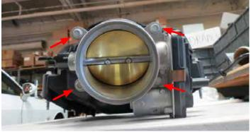
79. Using the supplied gasket and four (4) M6 x 40mm hex flange bolts from Bag #3, secure the throttle body to the supercharger inlet. Reconnect the electronic throttle body connector to the throttle body.
