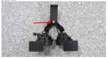
102. Install the horn assembly in the factory location using the factory bolt. Reconnect the horn connectors.
