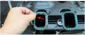
71. Clean and inspect the O-ring gaskets. Replace torn or damage O-rings as needed. Using a razor blade remove the tips off all eight (8) factory O-ring gaskets.
