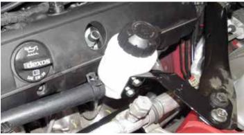
96. Route the LTR to Manifold hose through the hole in the radiator shroud and back towards the manifold. Using a 3/4" hose clamp from Bag #2, secure the hose to the upper barb of the LTR.
