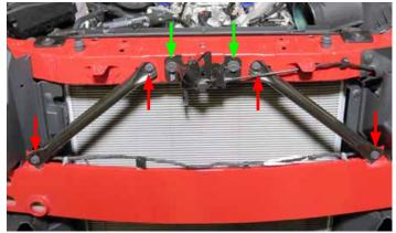
83. Disconnect and remove the horn assembly from the crash beam using a 10mm socket. Using a panel puller, remove the push pins securing the wire harness to the crash beam as well as the radiator shrouds.
