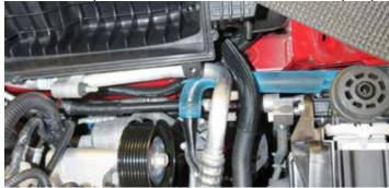
93. Remove the bolt securing the brace to the strut tower. Secure the surge tank to the surge tank bracket with two (2) M6 x 10mm bolts. Using factory bolt and supplied M8 x 25mm bolt, loosely secure the surge tank bracket to the brace. This will be removed again later in the install for the coil cover install.
