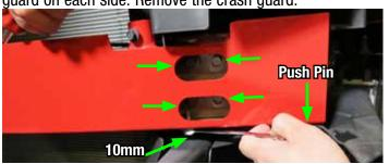
85. Using a panel puller, remove two (2) push pins securing the driver side radiator shroud to the radiator and one securing the rubber shroud. Remove both shrouds. The inner rubber shroud will not be reused.
