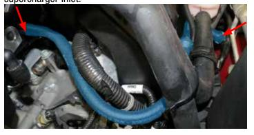
107. Connect the supplied EVAP hose to the hardline on the firewall at the rear passenger side of the manifold. Route the hose along the driver side of the manifold, beneath the coil wires, and connect it to the EVAP solenoid.
