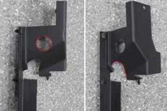
87. Reposition the shroud, and secure using the factory upper and vertical push pins.
