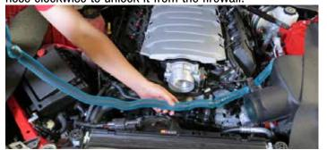
17. Disconnect the electronic throttle body connector from the throttle body.
