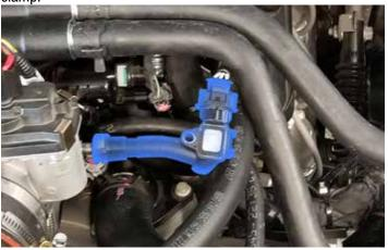
77. Using a breaker bar, rotate the tensioner counterclockwise and install the supercharger belt using the routing diagram below.
