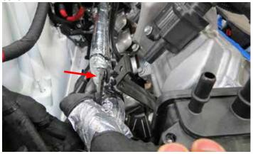
40. Using a 10mm socket, remove the engine harness support bracket. This bracket will not be reused.
