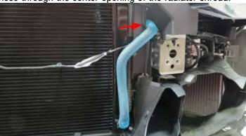
92. Secure the lower portion of the LTR to the air ducts using two (2) M6 x 16mm bolts and two (2) M6 locknuts from hardware Bag #2.
