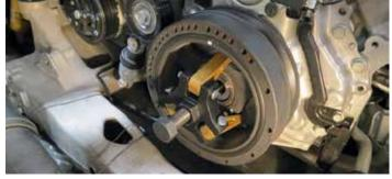
48. Apply white grease to the snout of the crank and to the inside of the balancer hub. Apply clean engine oil to the outside of the balancer hub.
