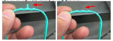
72. Install eight (8) modified 0-ring gaskets onto the runners.
