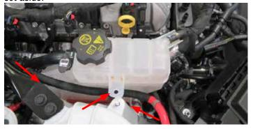
39. Using a panel puller, remove the engine harness from the support bracket located on the passenger side valve cover.
