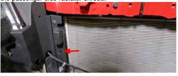
89. Using a panel puller, remove both inner push pins securing the right and left air ducts.
