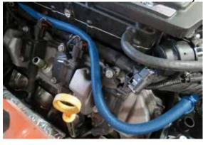
109. Connect the TMAP harness to the TMAP sensor located on the driver side of the manifold.
