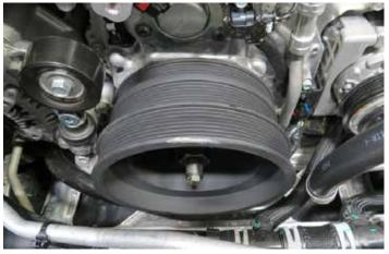
50. Using a 24mm socket and a torque wrench, install the used factory balancer bolt and torque it to 240 ft-lbs. Then remove the factory balancer bolt and discard.
