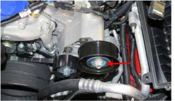
67. Install the smooth idler pulley to the upper water pump provision and the smaller grooved idler to the lower water pump provision. Torque both bolts to 22 ft-lbs.
