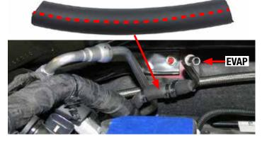
69. Connect the supplied fuel feed line to the hard line on the firewall and route it over towards the fuel adapter line. Secure the fuel line to the brake line with wire ties.
