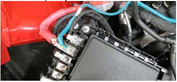
120. Remove the factory GROUND terminal nut attached to the chassis. Attached the GROUND connector on the water pump harness to the chassis ground and secure with the factory terminal nut. Remove the nuts securing the fuse box to the chassis. Gently remove the fuse box from the mounting studs and secure the relay to the mounting stud. Reinstall fuse box nuts.
