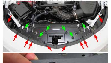
3. Using a 7mm socket, remove the bolts securing the bottom of the fascia.
