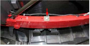
103. Reinstall the coolant reservoir tank, the electric fan assembly, and the radiator hoses. Replace the lower radiator tray.
