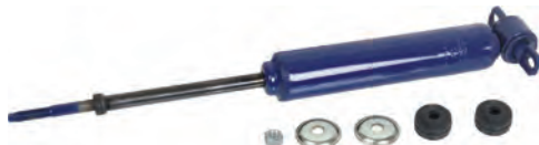
57-59 Heavy-duty, MONRO-MATIC PLUS , Ford and Mercury (2 required) ..... B7A-18124-M Δ 40.99 ea.
