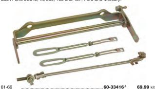
Includes all the linkage pieces for 2x4-barrel carburetor set-up: 9732, 9841 and 9B842, V8 406 and 427, low riser only, Ford and Mercury.
