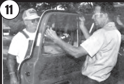
Install new division bar. Loosely attach with screws. Then re-install window regulator mechanism and door glass.
