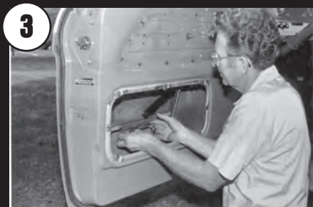
Release door glass from the regulator arm, leave in bottom of door. Take out after anti-rattlers are removed.
