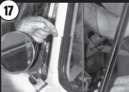
Pull cord out of groove in vent window rubber for tight overlapping fit of rubber to door.
