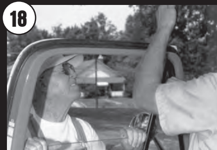
Hold glass while tightening vent window and division bar screws for best adjustment for glass.
