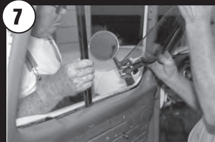
Release division bar then slowly remove vent window with a slanting inward and twisting-out motion.
