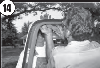
Working top right to left with a 3/8" wood strip, press clips in place. To prevent distorting curve section, do not press in.
