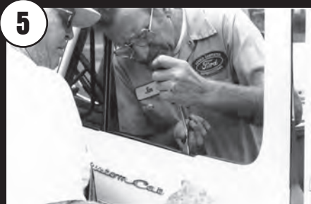
Pry anti-rattlers from door carefully then twist holding clips out with long-nose pliers. Then pull out door glass run.
