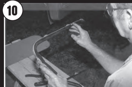
When installing new vent window rubber, check for indentations at correct location for pivot point on door.
