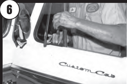
Remove various screws at top of door and under rubber holding vent window in place.
