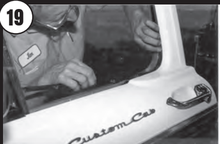
Anti-rattlers are the last new parts to install and can be snapped-in with a wood strip.
