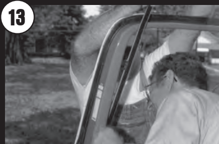
Glide new door glass run into position, fitting securely over edge of glass.
