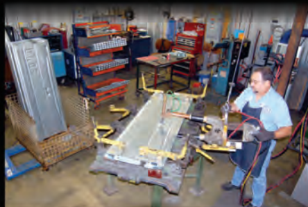
Welding original Ford tooling 1966-77 Bronco tailgates.
