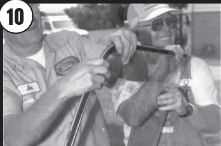
Use door window as a form for shaping curve in door glass run.
