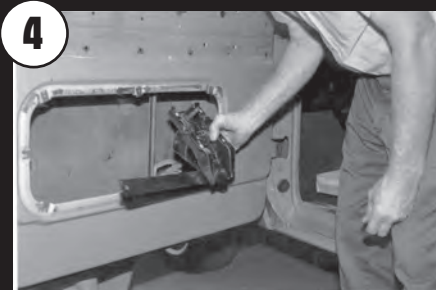
Removal of the window regulator mechanism will make removal of the division bar easier.
