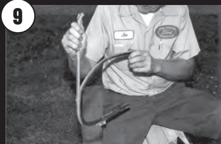
Old rubber pulls away easily from vent window.
