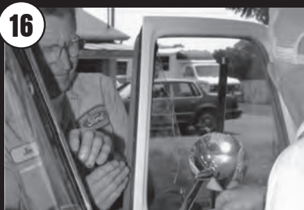
Re-install vent window, attaching screws loosely.
