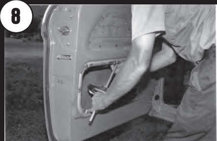
Division bar is a tight fit and requires patience to remove. Slowly twist while pulling outward.
