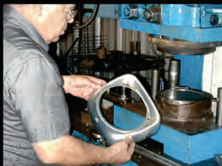
Seven stamping operations are required to make one 1961-66 F-100 headlight bezel.
