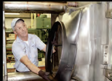
A 500 ton plastic injection machine is used to make larger parts such as fan shrouds and door panels
