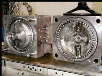
An opened injection mold used for making 1974-77 F-100-350 steering wheels
