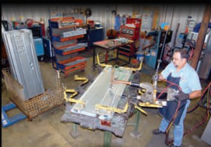
Welding original Ford tooling 1966-77 Bronco tailgates.
