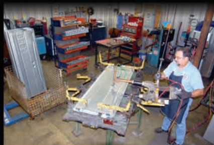
Welding original Ford tooling 1966-77 Bronco tailgates.
