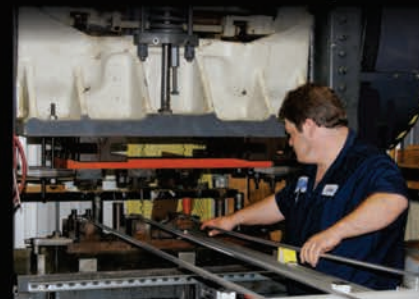
This press is fitted with a 3-stage progressive stamping die that makes 1977-79 F-100 race-track moldings.
