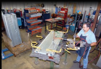
Welding original Ford tooling 1966-77 Bronco tailgates.
