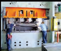
Metal stamping operations to make bumpers, hub caps, scuff plates
