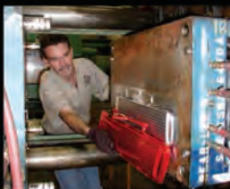
Plastic injection molding to make light lenses, emblems, fan shrouds,
