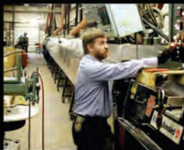
Rubber extruding operation to make door / trunk weatherstripping
