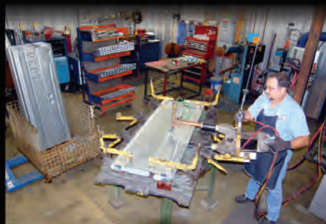
Welding original Ford tooling 1966-77 Bronco tailgates.
