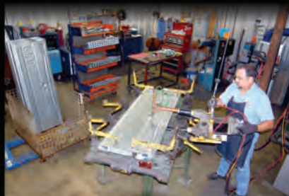
Welding original Ford tooling 1966-77 Bronco tailgates.
