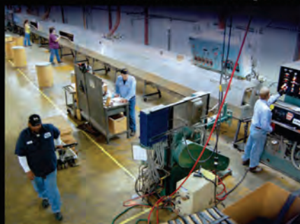
Our rubber extrusion machine extends 92' and is capable of producing 25,000' of weatherstripping daily.
