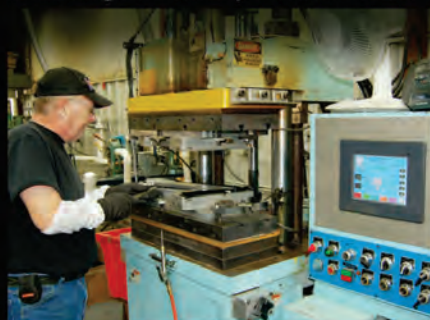
Rubber injection presses are used at Carpenters to make vent window seals and other molded rubber parts.
